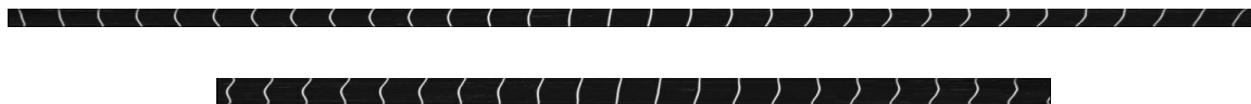
Figure 4.4: The results of changing the aspect ratio of the image in Fig. 4.3 by a factor of 50 in both the horizontal (top) and vertical (bottom, rotated 90 degrees) directions. This extreme change in aspect ratio makes it possible for a human observer to readily examine the pattern of lens distortion.
