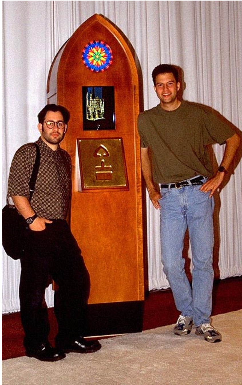
Figure 8.2: The Rouen Revisited kiosk, shown with the artists Golan Levin (left) and Paul Debevec (right). The brass plate in the middle of the kiosk is a touch pad that lets the user control the angle of view, time of day, amount of fog, and the rendering mode of the cathedral façade. The three rendering modes let the user view the cathedral as it appears in 1996, as it appeared in 1894 at the time Monet's paintings were made, or as it would appear with a Monet painting projected onto the cathedral's 3D geometry. The kiosk design and construction were done with the help of Warren H. Shaw, David Kaczor, Shane Levin, Joe Ansel, Charles "Bud" Lassiter, Scott Wallters, Chris Seguine and Bernie Lubell.
