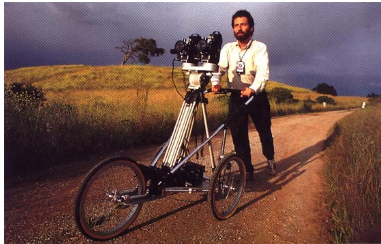
Figure 1.3: The Immersion '94 stereo image sequence capture rig, being operated by Michael Naimark of Interval Research Corporation. Immersion '94 was one project that attempted to create navigable, photorealistic virtual environments from photographic data. The stroller supports two identical 16mm movie cameras, and has an encoder on one wheel to measure the forward motion of the rig. The cameras are motor-driven and can be programmed to take pictures in synchrony at any distance interval as the camera rolls forward. For much of the work done for the See Banff! project, the forward motion distance between acquired stereo pairs was one meter. Photo by Louis Psihoyos-Matrix reprinted from the July 11, 1994 issue of Fortune Magazine.
