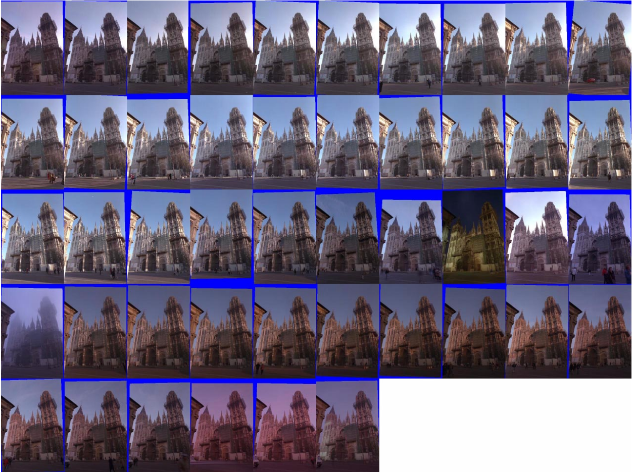
Figure 8.7: This series of photographs shows the entire set of photographs taken from the alpha camera location over the period of January 14-16, 1996. The images have all been digitally rectified so that cameras all have the same rotation as well as position. As a result, any one of these time-of-day photographs can be projected onto the model using the camera pose information from the master alpha image. The beta and gamma series of images were similarly processed.
