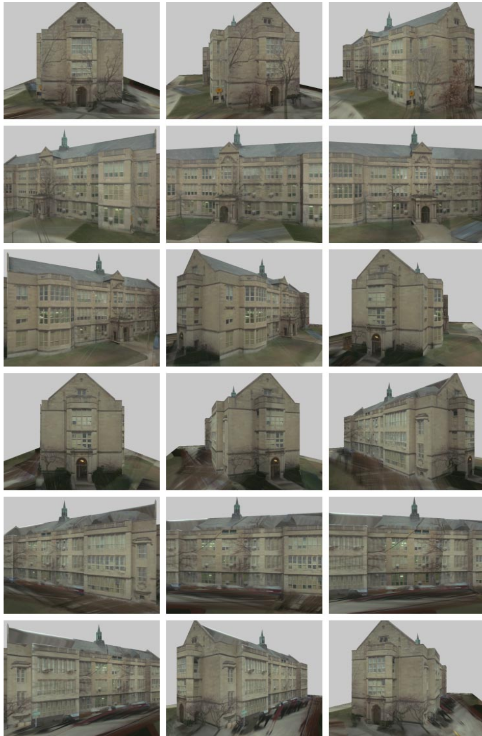
Figure 6.6: University High School fly-around, with trees. This sequence of images shows every twentieth frame of a 360-frame fly-around of the building, using twelve photographs to texture-map the model with view-dependent texture mapping.
