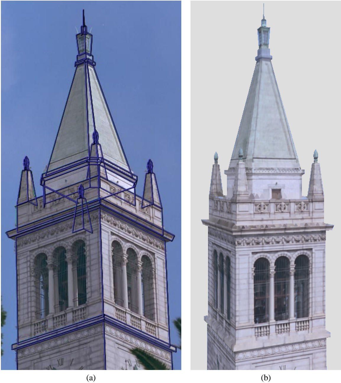
Figure 5.2: (a) The accuracy of the model is verified by reprojecting it into the original photograph through the recovered camera position. (b) A synthetic view of the Campanile generated using the view-dependent texture-mapping method described in Section 6. A real photograph from this position would be difficult to take since the camera position is 250 feet above the ground.
