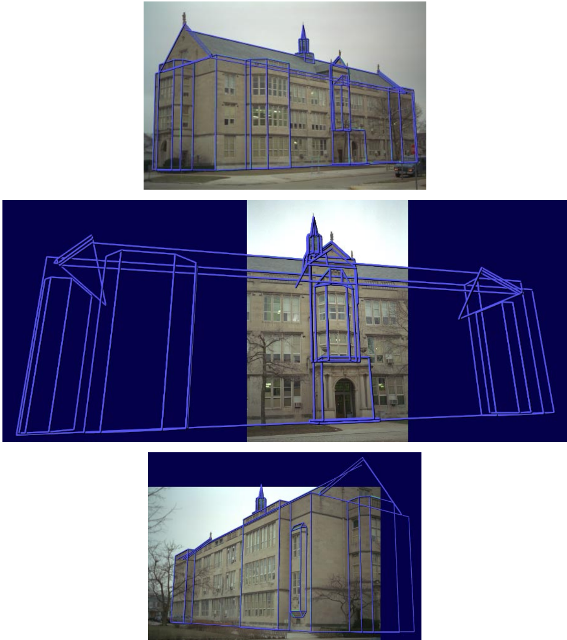
Figure 5.13: The edges of the reconstructed model, projected through the recovered camera positions and overlaid on the corresponding images. The recovered model conforms to the photographs to within a pixel in all twelve images, indicating that the building has been accurately reconstructed.
