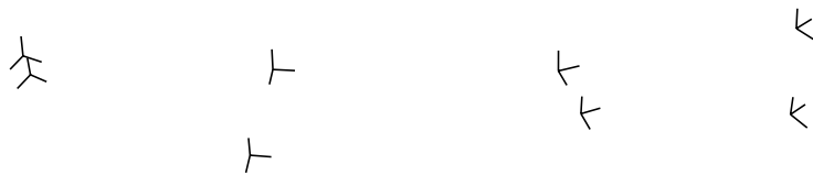
Figure 2.2: Images from the 1995 Taylor-Kriegman structure from motion paper [47]. In this work, structure from motion is recast in terms of line segments rather than points. A principal benefit of this is that line features are often more easily located in architectural scenes than point features. Above are two of eight images of a block scene; edge correspondences among the images were provided to the algorithm by the user. The algorithm then employed a nonlinear optimization technique to solve for the 3D positions of the line segments as well as the original camera positions, show below. This work used calibrated cameras, but allowed a full perspective model to be used in contrast to Tomasi and Kanade [50]. However, the optimization technique was prone to getting caught in local minima unless good initial estimates of the camera orientations were provided. This work was extended to become the basis of the photogrammetric modeling method presented in Chapter 5.
