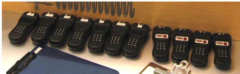
Electronic Voting Wands, labeled with the jurors' names. 3M "Privacy-Guard" film seen on the left group of units prevented the displayed numeric vote values from being easily seen by others.
